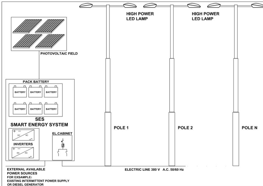
The Grid-connected solution involves the installation of single poles equipped with LED lamps or, alternatively, using the existing poles in which the traditional lamp is replaced with LED technology.
