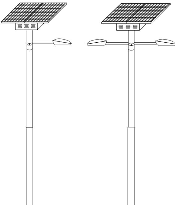
The Stand-alone solution involves the installation of individual poles equipped with solar panels, storage batteries, electronic control system and LED lamp.
